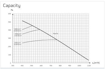
Max Pa capacity of standard unit, Pt, ext as a function of qv, to SFP-values. Acc. to EN13053 for a unit with filters, no heating element. Airflow speed above evaporator is measured at meters per second.
