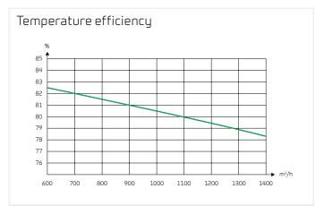
Temperature efficiency for units with counterflow heat exchanger according to EN308 (dru)
