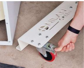
Step 4 Tilt unit and hook locked wheels under cylinder side
