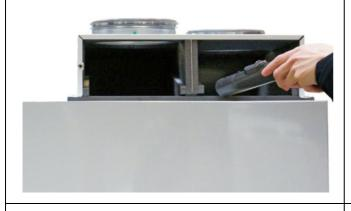
Remove the filter material from their trays. Wash in a basin of water or in a cool cycle of a washing machine and dry.
