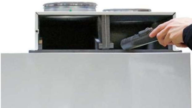
Remove the filter material from their trays. Wash in a basin of water or in a cool cycle of a washing machine and dry.
