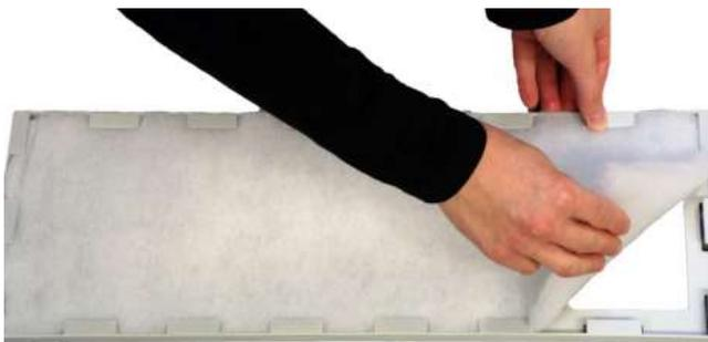
Once held in place by the tray edges, slide them back into the filter box, screw door closed and turn on again.
